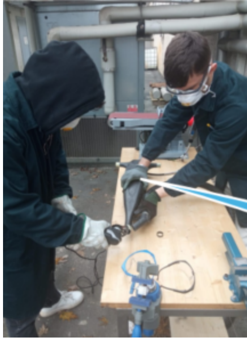
Figure 7. Surface finishing and final weigh-in. Measured mass \approx 477 g against a 480 g target.
